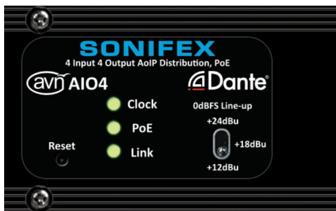
Fig 2-2: AVN-AIOx Indicators and Reset
