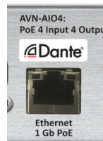
Fig 2-14: Ethernet/PoE Connection (AIO4/AIO8/AI16/AO16/AESIO8)
